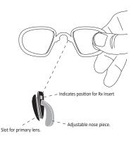
The prescription insert is held in place by aligning the buds on the Rx Insert into the notches on the nose piece.
