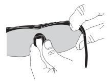
Ballistic spectacles protect best when the entire perimeter of the lens and frame are closest to the wearers face. For your best, most protective fit, adjust the nose piece so that there is minimal gap between the lens, the side of your face and under your eyes.
