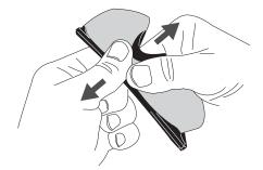
Position one hand to grasp the frame at the center of the brow bar, the other hand directly opposite at the nose piece lens junction, as pictured. Simply pull apart.
